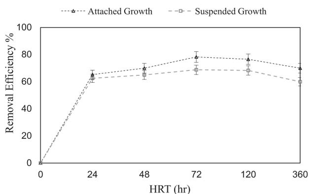
Fig. 1. BOD<sub>5</sub> removal efficiency in suspended and attached growth.
