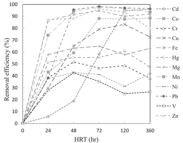
Fig. 5. Heavy metal removal efficiency in suspended growth system.
